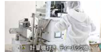
Tea packing machine with weighing mechanism
